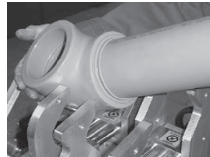
Fig. 12 Remove the welding joint after the end of the cooling time from the clamping jaws
