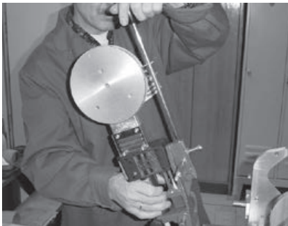
Fig. 1 Set the heat reflector in the holder
