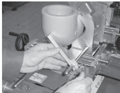
Fig. 7 Adjust the stop to hold the fittings
