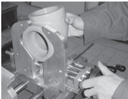
Fig. 6 Place and adjust the fitting in the clamping jaw
